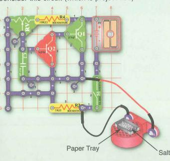
This circuit can be used to demonstrate how a speaker creates sound using mechanical vibrations. Connect the speaker using the jumper wires and lay on a table. Using paper, scissors, and tape, make a small tray and lay on the speaker, as shown. Here is a sample cutout pattern:
