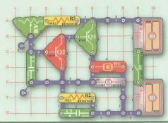
The frequency (pitch) of the sound is controlled by the resistors and capacitors in the circuit, increasing their values decrease the frequency. One way to change it is using the adjustable resistor. Another way is to place the  $0.1\mu F$  capacitor on top of the  $0.02\mu F$ , increasing the capacitance (project 200). You could also replace the  $100k\Omega$  resistor with the photoresistor to control the frequency using light.
