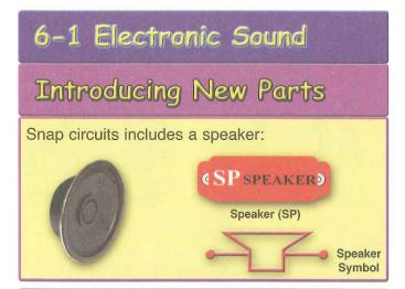
A **speaker** converts electricity into sound. It does this by using the energy of a changing electrical signal to create mechanical vibrations (using a coil and magnet similar to that in the motor). These vibrations create variations in air pressure, called sound waves, which travel across the room. You "hear" sound when your ears feel these air pressure variations.
