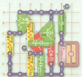
In this circuit the red LED will be flashing, the flash rate is controlled by the adjustable resistor. Although the LED might appear to be solid at the highest setting of the adjustable resistor, it is actually flashing at a faster rate than your eyes can see. Here the LED flash rate can be adjusted from less than once a second up to 30 times a second. This flash rate is called the frequency.
