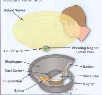
A speaker can only create sound from a CHANGING electrical signal, for unchanging electrical signals it acts like an  $8\Omega$  resistor. (An unchanging signal does not cause the magnet in the speaker to move, so no sound waves are created).
